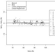
This graph shows plots of the error  $(SpO_2 - SaO_2)$  by  $SaO_2$  using the 9550 with a linear regression fit and upper 95% and lower 95% limits of agreement. Each sample data point is identified by subject from a clinical study in non-motion conditions.
